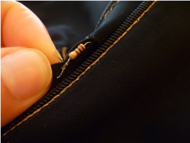
Fig. 6: resistor sewn with conductive thread
